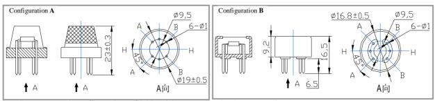
Structure and configuration of MQ-135 gas sensor is shown as Fig. 1 (Configuration **A or B**), sensor composed by micro AL<sub>2</sub>O<sub>3</sub> ceramic tube, Tin Dioxide (SnO<sub>2</sub>) sensitive layer, measuring electrode and heater are fixed into a crust made by plastic and stainless steel net. The heater provides necessary work conditions for work of
