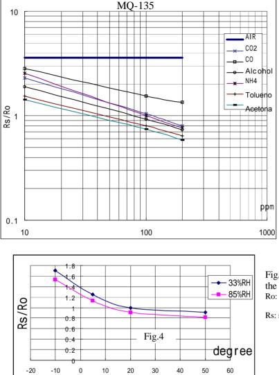
Fig.3 is shows the typical sensitivity characteristics of the MQ-135 for several gases. in their: Temp:  $20^{\circ}C_{\gamma}$  Humidity:  $65\%_{\gamma}$  O<sub>2</sub> concentration 21% RL= $20k \Omega$ Ro: sensor resistance at 100ppm of NH<sub>3</sub> in the clean air.
