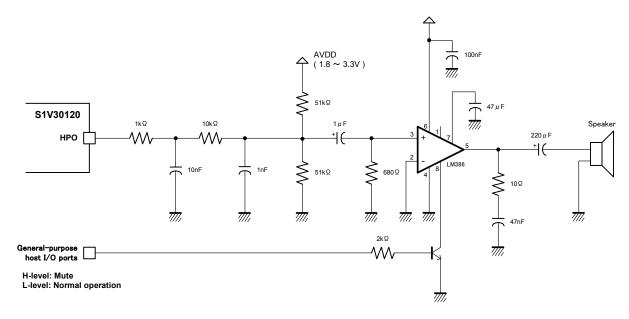
Figure 3.1 Example of full-digital amplifier add-on circuit using a linear op-amp
