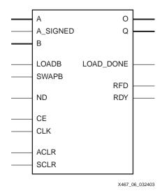
Figure 8: Core Multiplier Generator Symbol
