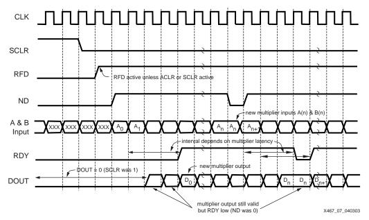
Figure 9: Multiplier Generator Timing Diagram
