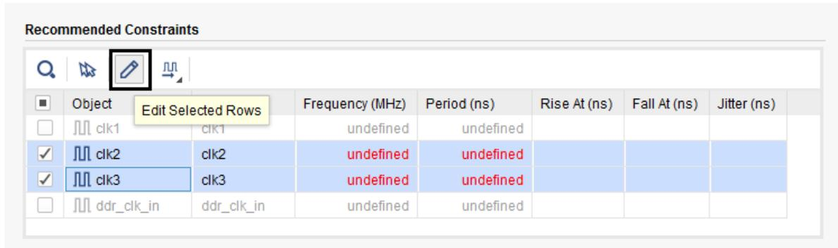
Next, fill out any required fields, such as Frequency and Period as shown in the following figure:
