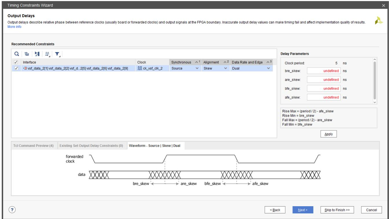
After you select the proper template, you must enter the delay parameters values. To accelerate the delay parameter entry task, you can select and edit several constraints with same clock and same template at once. After the constraints have been completed and applied, you can review their corresponding Tcl syntax in the Tcl Command Preview tab or you can click **Next** to proceed to the next step.
