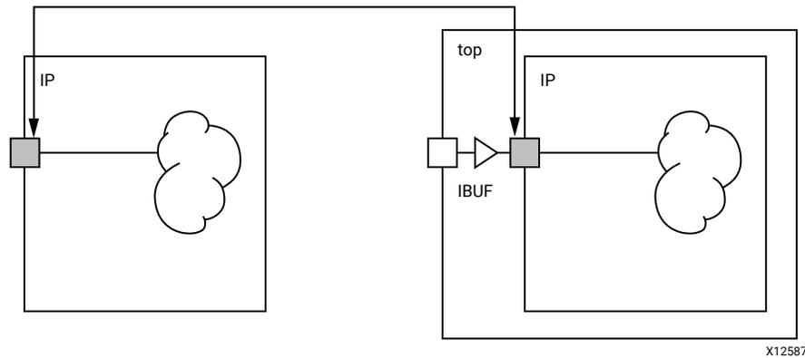
This capability is very useful for creating constraints on the interface of an IP or a sub-level module without knowing the names of the top-level design.
