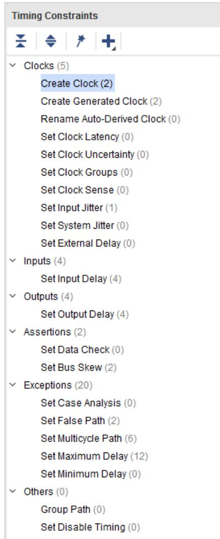
To create a new constraint, double click the name of the target constraint. A dialog box allows you to specify the value for each option. When you click **OK**, the tool does the following:
