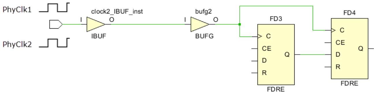
While their overlap is convenient for timing several application modes with one design and constraint database, these clocks and their children generated clocks should never be timed together. The Timing Constraints wizard identifies such clocks and recommends a clock groups constraint to prevent unnecessary timing analysis on the clock domain crossing paths, as shown in the following figure.
