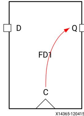
If the constraint is applied to FD1/Q, the timing engine stops the propagation through the arc C->Q to make the pin Q a valid startpoint:
