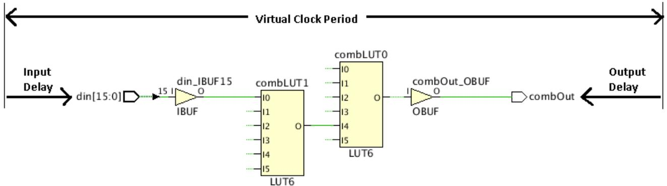
The final combinational path delay constraints are:
