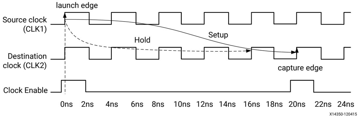
With a four-cycle hold requirement, the timing-driven implementation tools usually have to insert a large amount of delay in the datapath in order to meet hold timing in both Slow and Fast timing corners. This results in unnecessary area and power consumption. For this reason, it is important to relax the hold requirement when possible.
