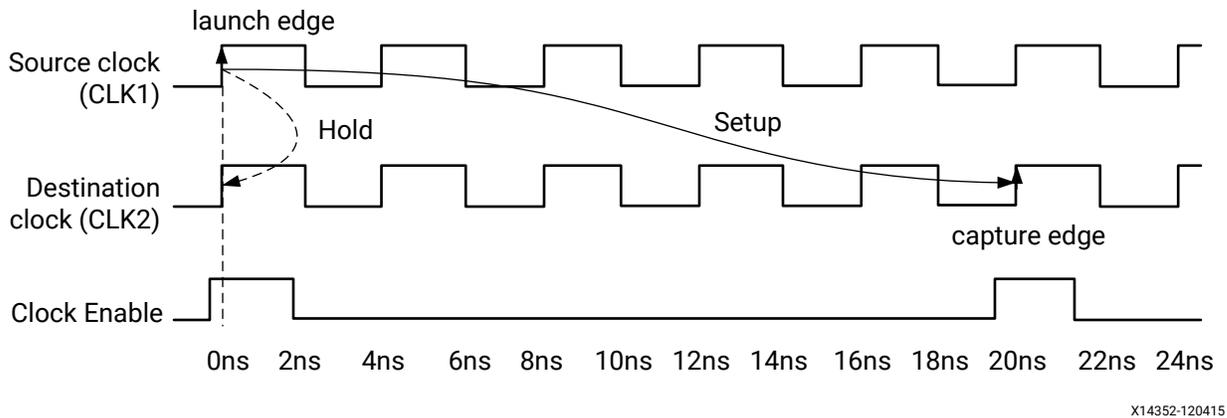
★ **IMPORTANT!** In general, within a clock domain or between two clocks with the same waveform, when a setup multiplier of  $N$  is defined, define a hold multiplier of  $N-1$  (most common case) as shown below.
