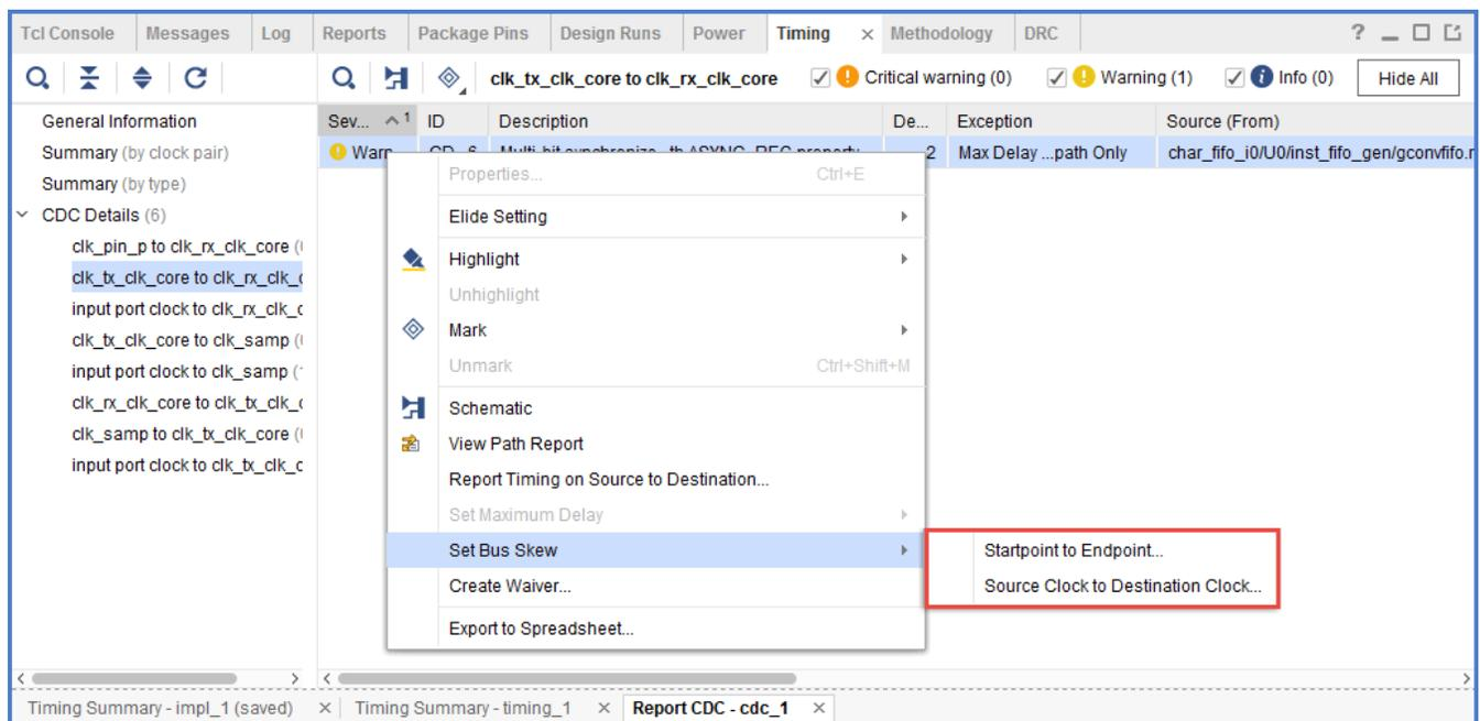
**Note:** Vivado does not verify the validity of setting a bus skew constraint on the selected objects. You must ensure that a bus skew constraint makes sense with the selected objects.
