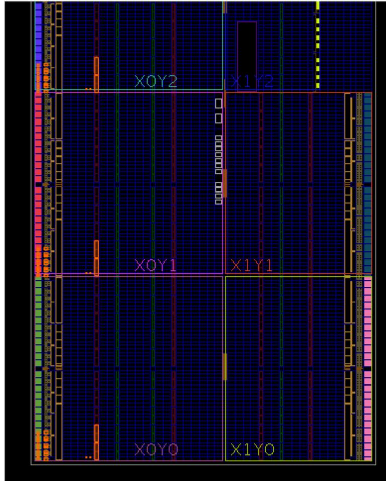
To determine absolute grid RLOCs, use the site RPM\_X and RPM\_Y properties. For example, the lower block RAM is placed at site RAMB36\_X0Y0.
