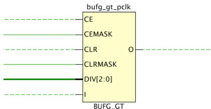
In such case, the tool assumes the worst possible scenario for the output clock (divide by 1) and propagates the incoming clock to the buffer output. This worst-case scenario might be pessimistic and over-constrain the design if a clock division of 1 is never exercised. It is possible to control the auto-generated clock on the BUFG\_GT output pin by setting the DIV[2:0] bus with a `set_case_analysis` constraint.
