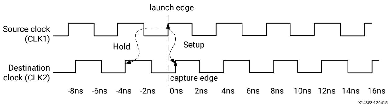
In this example, the setup constraint due to the phase-shift is 0.3 ns. This makes it almost impossible to achieve timing closure. On the other hand, the hold check is -3.7 ns, which is too lenient.
