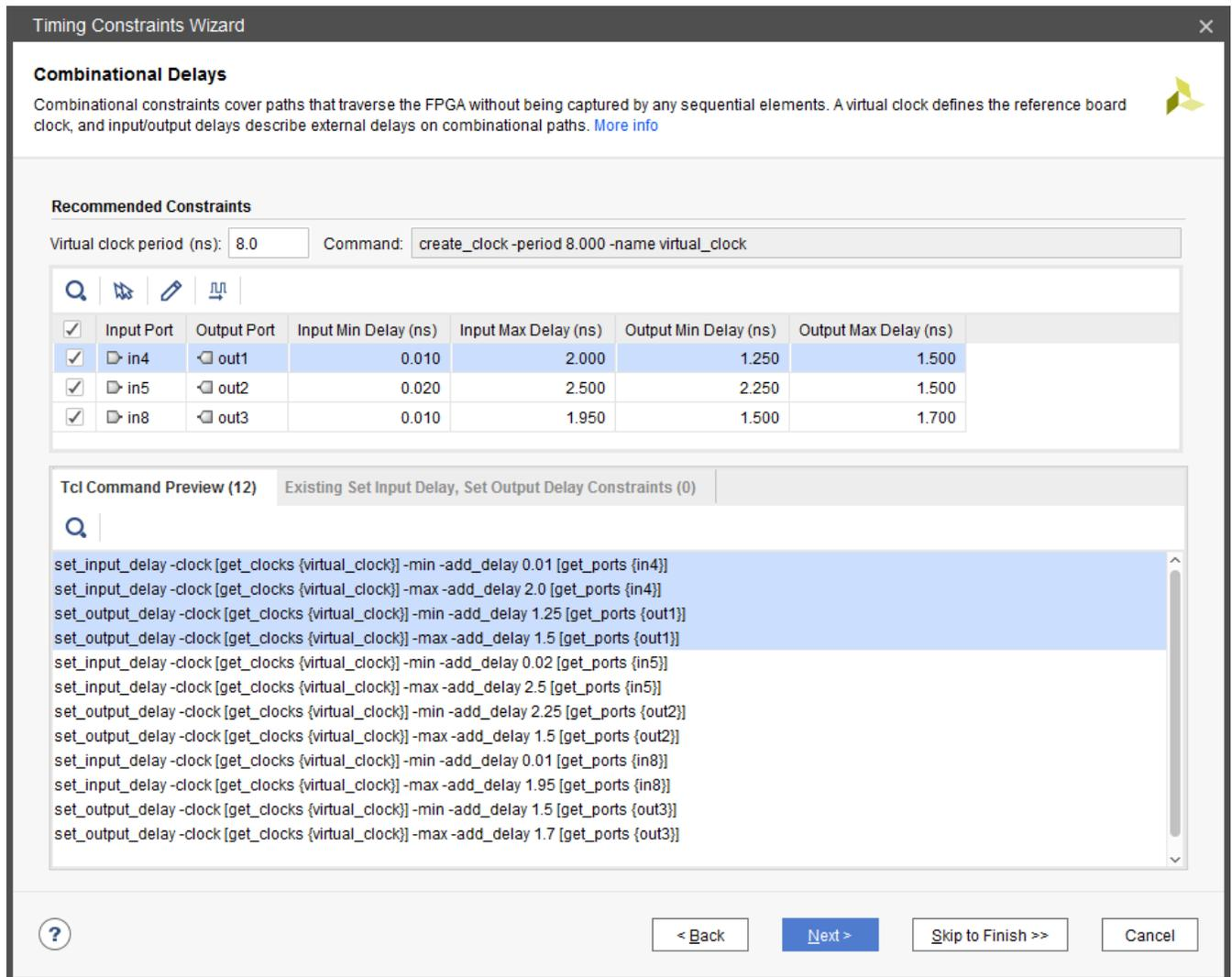
None of the input and output delay constraints override existing ones. If a given port has multiple delay constraints with respect to the same clock, the smallest value of all constraints is used by the Vivado Timing analysis feature during hold analysis, and the largest one during setup analysis.
