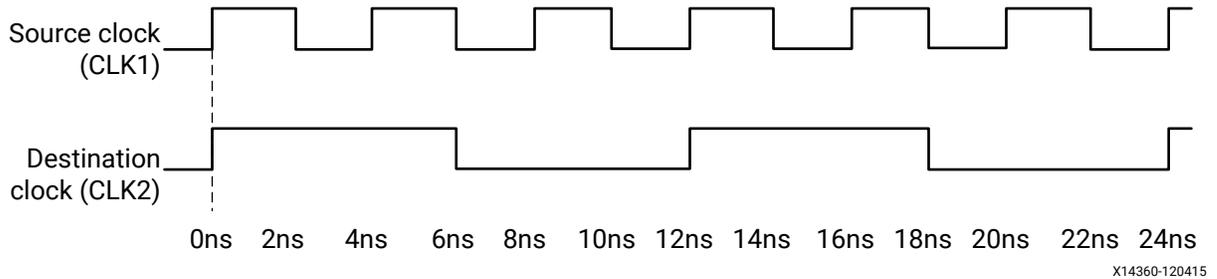
The setup and hold relationships that are resolved by the STA tool when no multicycle is applied are shown in the following figure:
