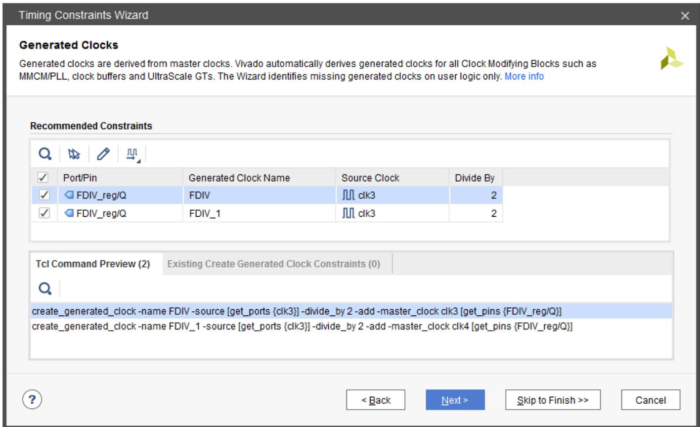
When several master clocks reach the generated clock source point, the wizard creates all the corresponding generated clocks, using unique names and clear reference to individual master clocks. The previous figure illustrates the scenario where two clocks (clk3 and clk4) reach the sequential cell FDIV\_reg. Consequently, two generated clock constraints (FDIV and FDIV\_1) are recommended.
