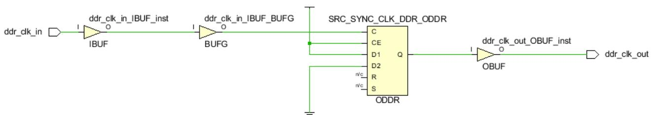
For the UltraScale device family, the ODDR and ODDRE1 primitives are automatically retargeted to OSERDESE3 with the property ODDR\_MODE=TRUE. The wizard recognizes the topology shown in the following figure, where OSERDESE3/D[0] is connected to 1 and OSERDESE3/D[4] is connected to 0 (no phase-shift).
