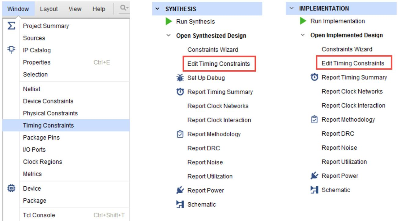
The Timing Constraints window displays the timing constraints in memory, in either the same sequence as in the XDC files and Tcl scripts, or the same sequence in which you entered them in the Tcl Console.
