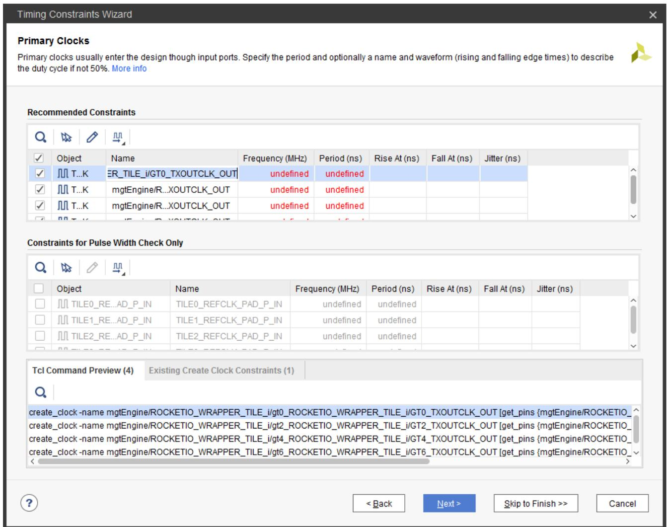
The screenshot shows the 'Timing Constraints Wizard' window. The 'Primary Clocks' section is active, displaying two tables of recommended constraints.
