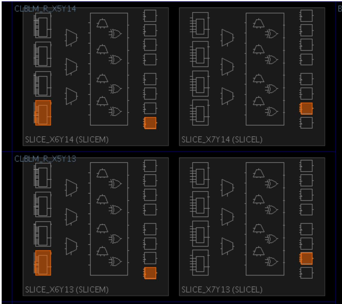
The macro contains SRLs which are based on LUTRAMs, and which can be placed only in SLICEM type slices. This places slight restrictions on the possible locations of the macro. The macro can be located only where a SLICEL column is to the right of a SLICEM column.
