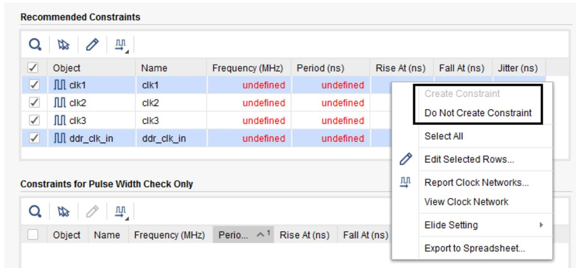
In the following figure, `clk1` and `ddr_clk_in` are unchecked and will be skipped.
