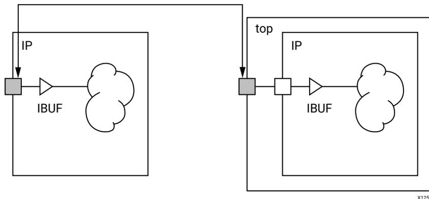
The following figure, the IP does not contain an I/O buffer, so the synthesis engine infers one between the IP interface pin and the top-level port. Consequently, the `get_ports` is converted to a `get_pins` of the IP interface pin (for example, a hierarchical pin) when the XDC is applied.
