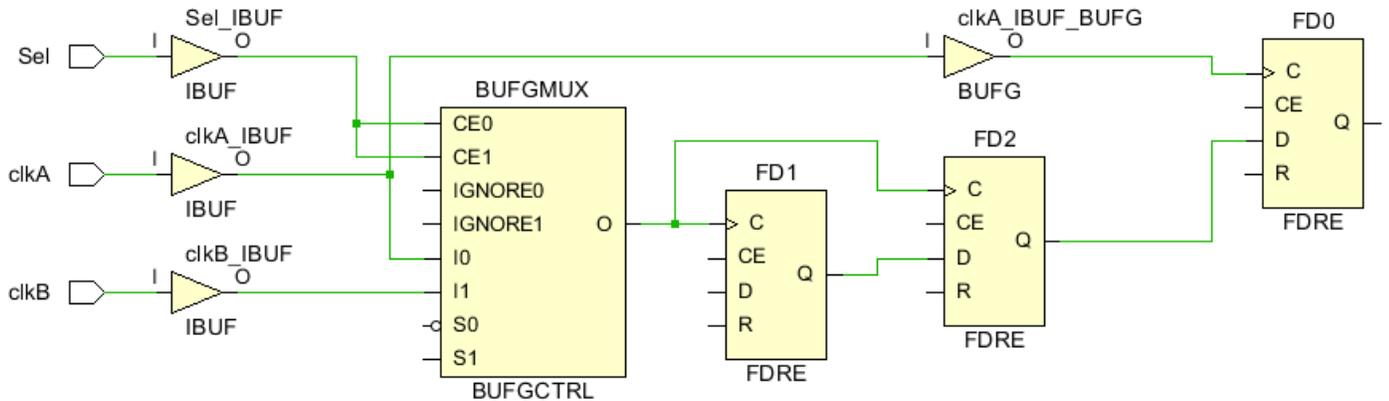
Because only the clock domain crossing paths of the shared clock tree must be ignored, the wizard recommends to create generated clocks that are copies of `clkA` and `clkB` but that only exist on the shared clock tree. The clock groups constraint is applied to the generated clocks only, so that the paths outside the logic of the shared clock tree can still be normally timed. The following figure illustrates the wizard recommended constraints for the example above.
