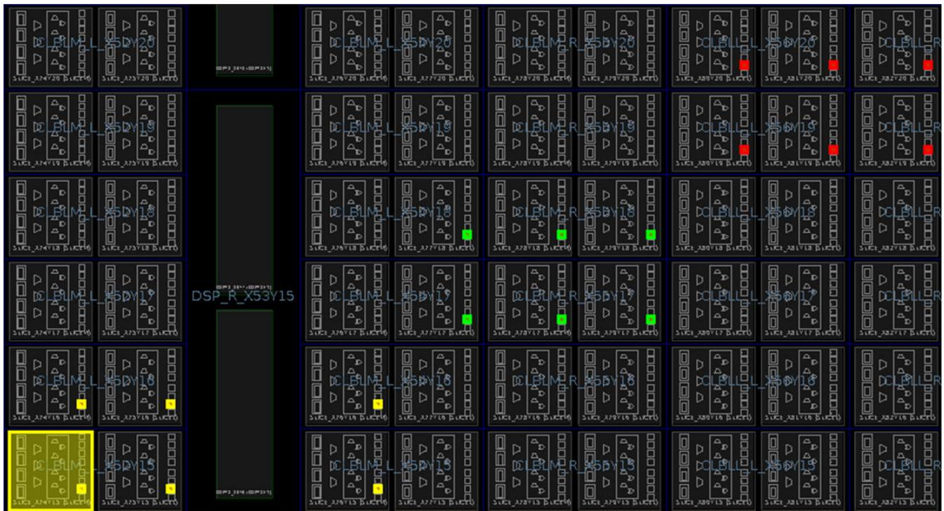
The following example shows a hierarchical RPM that is fixed using RLOC\_ORIGIN. RLOC constraints are assigned to the RPM register cells to create a two-up-by-three-across placement pattern.
