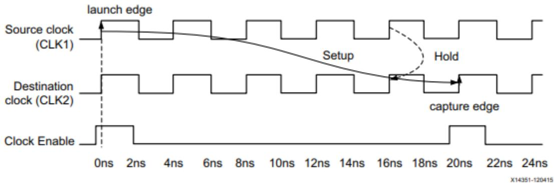
Because both source and destination clocks have the same waveforms, and are phase-aligned, Figure 66 is equivalent to Figure 67.
