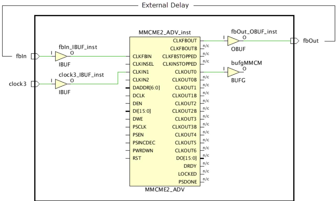
In the current Vivado Design Suite release, the Timing Constraints wizard cannot recommend external delay constraints when there is a sequential cell in the feedback path, such as ODDR, which is used for generating a forwarded clock. In this case, you must create the external delay constraints manually or using the Timing Constraints window after exiting the wizard.
