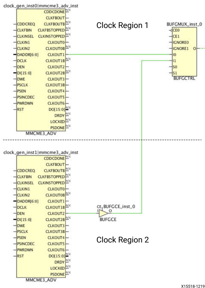
Figure 64: Routing the Clock to Another Clock Region
