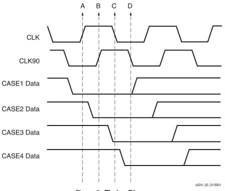
These waveforms are shown in the Figure 3 timing diagram along with the four possible data arrival cases used in the next section.
